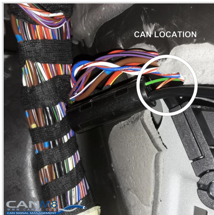
CAN Wiring in the driver door harness (Contactless Reder installed)
