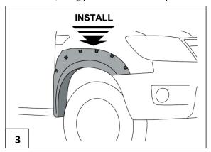
Fit the fender flare to the vecihle in the Uppermost vertical position before final fixings.
