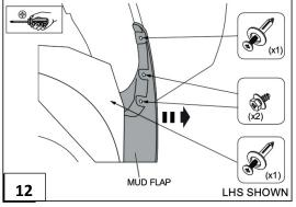
Remove the rear mud flaps by removing and retaining the screws and scrivets from inside the wheel arch as shown.
