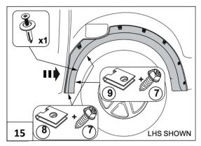
Attach the front part of the rear fender flare with (3) Hex head screws and speed nuts as per front fender process Reuse one factory plastic scrivet as shown.
