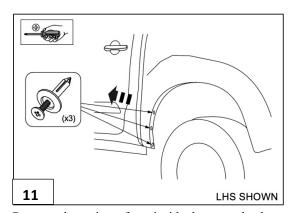
Remove the scrivets from inside the rear wheel arch as shown.
