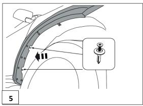
Reattach the wheel arch liner with factory scriyets.
