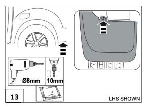
Carrefully drill though centre of rivet holding the liner behind the rear mud flap with a 8mm drill bit and 10mm drill stop as shown Carrefully
