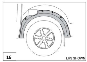
Ensure that flares are aligned. Remove the tape liner. contacting the vehicle surface around the full perimeter. Apply firm pressure on the flare to ensure the tape is of the flares.
