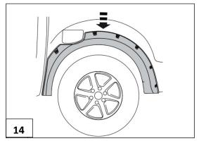
Fit the fender flare to the vehicle in the uppermost vertical position before final fixing and tape application is completed as shown
