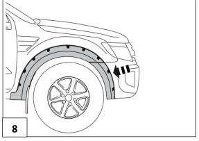
Fit the bumper flare to the vehicle as shown.
