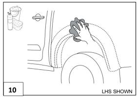
Wash the areas of contact on the vehicle and wipe the fender where the flare will contact using provided alcohol wipes.
