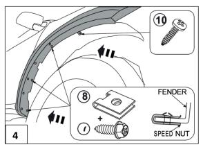
Hold the splash guard inwards and push the supplied. Speed nuts onto the front guard into the hole positions as shown. Fold the plastic Tab inwards over the fender and secure with one Philips head screw.
