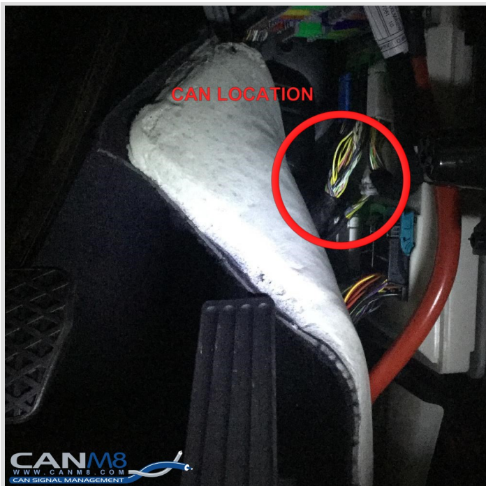
Body Domain Controller located behind the driver side kick panel
